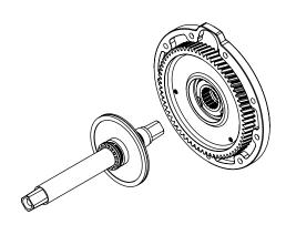
**3. Slide the remaining axle assembly in.**Note: Grease all touching surfaces to make for easy maintenance.
