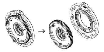
4. Screw 3 M4 screws\* into the back side of the drive gear until they are touching the bearing. Start turning one screw one turn, then the next screw once, then turn the next screw one turn, then the next. Repeat until the gear is removed.
