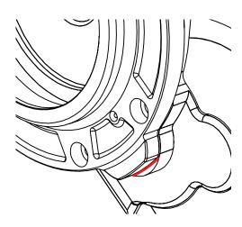
1. Place the Lekkie Drive Cover HD on the motor and trace the cover edge on the pinion housing as shown.
