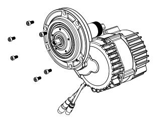
4. Install paper gasket then slide the new drive assembly into place. Clean, apply Loctite 243, and install the six M5 drive cover bolts. Tighten to 6Nm.
