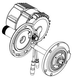
2. Tap the axle from left side of motor, loosening the drive assembly and remove assembly.
