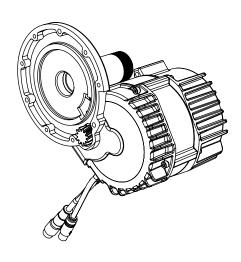
2. Remove the Lekkie Drive Cover HD. Note the scribed mark showing the material you will be removing.
