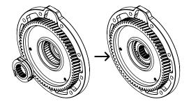
1. Press the main drive gear into the new bearing in the Lekkie Drive Cover HD.
