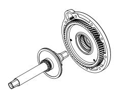
3. Holding the stock drive cover, gently tap the axle from the drive side and pull out the axle assembly.
