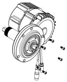
1. Using a 4mm hex/allen unscrew the six screws holding on the stock cover and remove.
