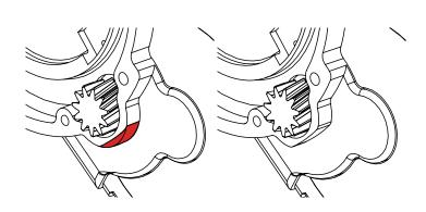
3. Using a file, carefully remove material up to the scribed in line, making it the same shape as the Lekkie Drive Cover HD. You may also need to trim the paper gasket to fit (this may be done after assembly).
