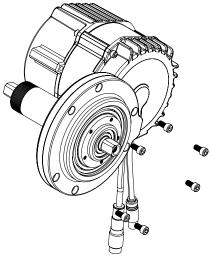
1. Using a 4mm hex/Allen key unscrew the six screws holding on the stock cover and remove.
