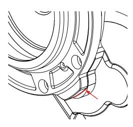
1. Place the Lekkie Drive Cover HD on the motor and mark the edge of the cover, scribing onto the motor housing in the area shown.
