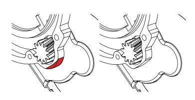
3. Apply tape/masking over the drive gears/ opening to avoid metal filing contamination inside the motor.
