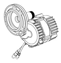
4. Place the Lekkie Drive Cover HD on the motor and check the shape. Repeat previous steps if more material removal is required.
