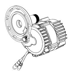
2. Remove the Lekkie Drive Cover HD. Note the scribed mark showing material requiring removal.
