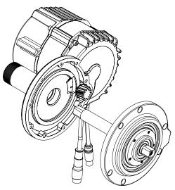
2. Tap the axle from left side of motor, loosening the drive assembly and remove assembly.
